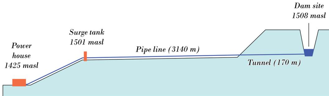
Fig. 2: Hydraulic scheme of BTHPP.
