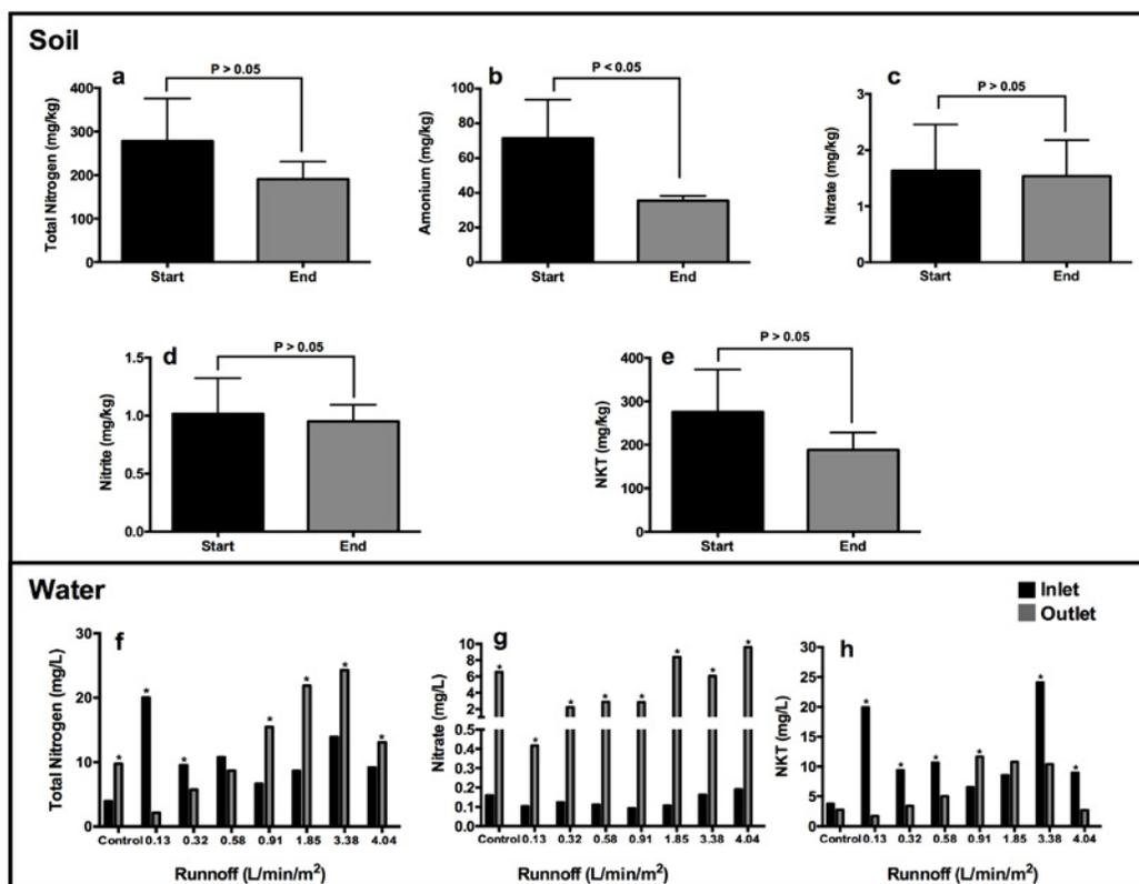
Figure 3. A plot of the concentration of nitrogen compounds in the soil (a, b, c, d, and e) and water (f, g, and h).
