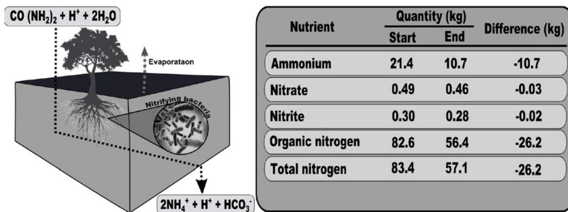
**Figure 4.** Mass balance of the nitrogenous compounds in the rain garden.
