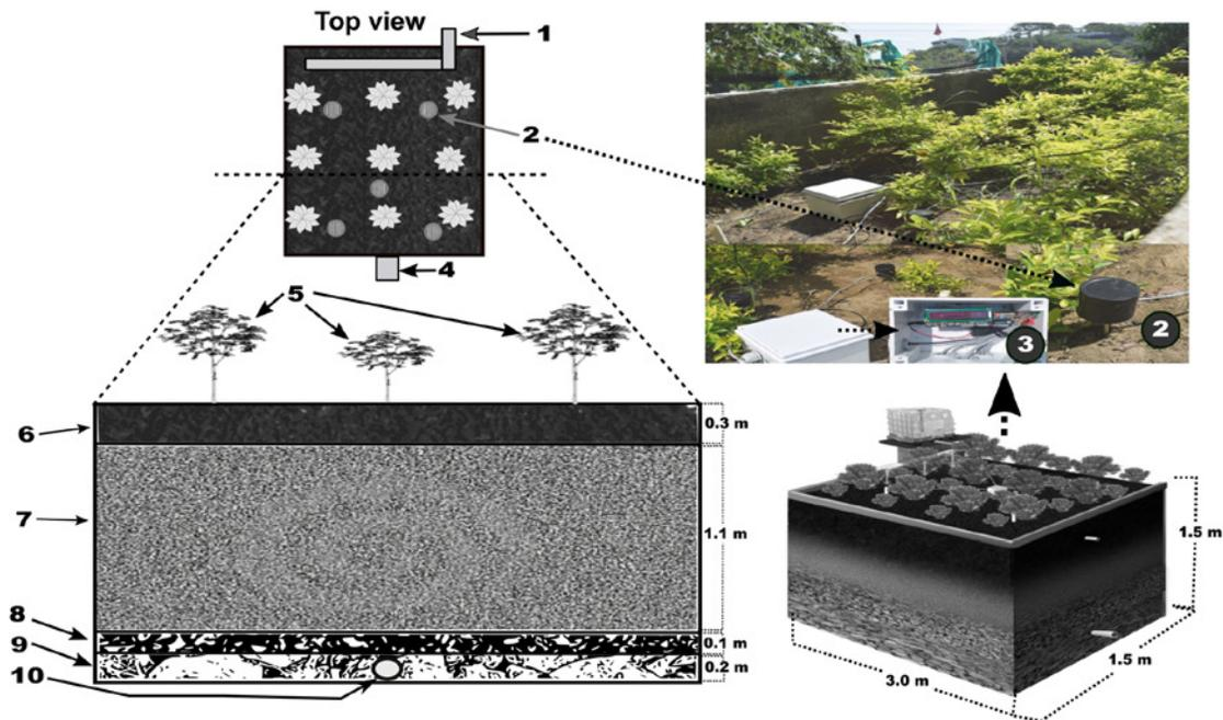
**Figure 1.** Rain garden components: 1. Affluent; 2. Automatic monitoring sensors (pH, humidity and temperature); 3. An Arduino sensor for collected data processing; 4. Effluent; 5. *Duranta golden* specimens (density: 5 specimens/m<sup>2</sup>); 6. Organic fertilizer superficial layer; 7. Sand layer (0.075 mm – 0.5 mm); 8. Fine gravel layer (5-20 mm); 9. Coarse gravel layer (20-80 mm); 10. Outlet pipe.
