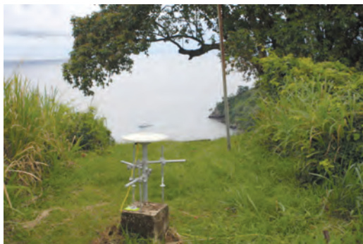
Fig. 2. Geodetic monument occupied at Chatham Bay in 1991 and 2008 (left). View from Chatham Bay showing location of geodetic monument of campaign site COCO (right).
