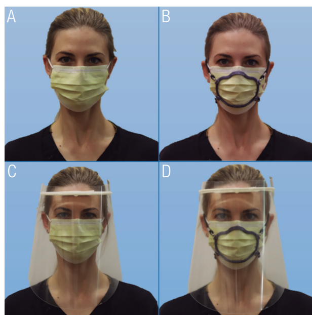
Figure 1. Different scenarios of the sample characterization. A=Group 1: mask only (M); B= Group 2: Mask+frame (MF); C= Group 3: Mask+face shield (MFS); D= Group 4: Mask+frame+ face shield (MFFS).
