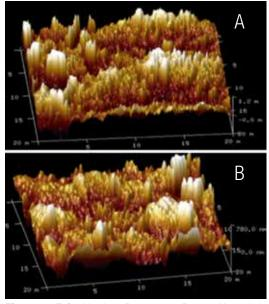
**Figure 3:** ZrO<sub>2</sub> Absolute Roughness (Ra): a) Monoclinic phase showed a higher topographic roughness (Ra. .320  $\mu$ m) at natural state. b) Tetragonal phase showed a lower roughness (Ra .126  $\mu$ m) after sintered process. The monoclinic phase has a greater roughness but cannot be used as a trans-endodontic implant.
