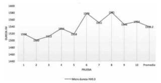
**Figure 5.** Vickers ZrO<sub>2</sub> tetragonal microhardness: load: 2.942N (300 gr) for 15 seconds, 10 indentations. The result of the sum of the indentations was 1500 HV.
