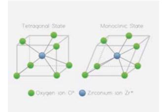
**Figure 1.** Zirconium oxide phase transformation. Phase change of the ions of zirconium oxide and oxygen in monoclinic phase, and subsequent to the sintered the tetragonal phase.
