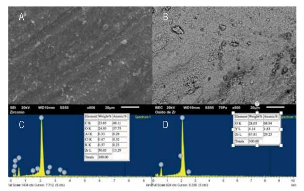
**Figure 4**. SEM/EDS analysis. SEM a) SEM image of ZrO<sub>2</sub> in monoclinic phase, x800 objective, b)SEM image of ZrO<sub>2</sub> in tetragonal phase, final process after sintered treament at 1170°C. c) EDS analysis showed the compounds of ZrO<sub>2</sub> in monoclinic phase. d) EDS final compounds of ZrO<sub>2</sub>.
